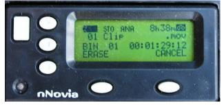
• Press the Left Selection button ("ERASE") to clear the bin. The Recording Clock goes to 00:00:00:00 to show the bin is empty. Press the Menu button twice to exit.
