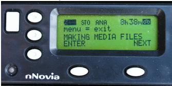
2) Press the Right Selection button ("NEXT") 6 times. The screen will display, **"SYSTEM SETUP"**)
