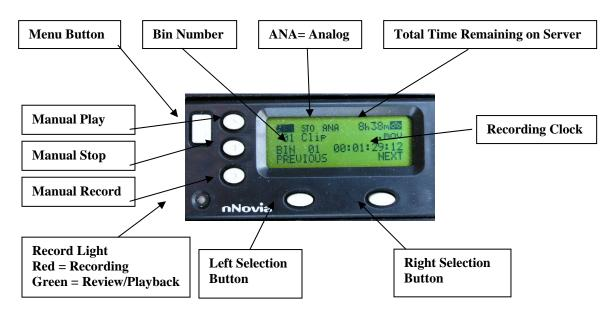
• **Manually Clear the Bin-** Occasionally, the video server will get out of synch with the processor causing video replay to malfunction. Clearing the bin will usually re-synch the two but be aware that this will obviously delete the entire clip. It is also recommended that the bin be manually cleared at the beginning of each competition day.
